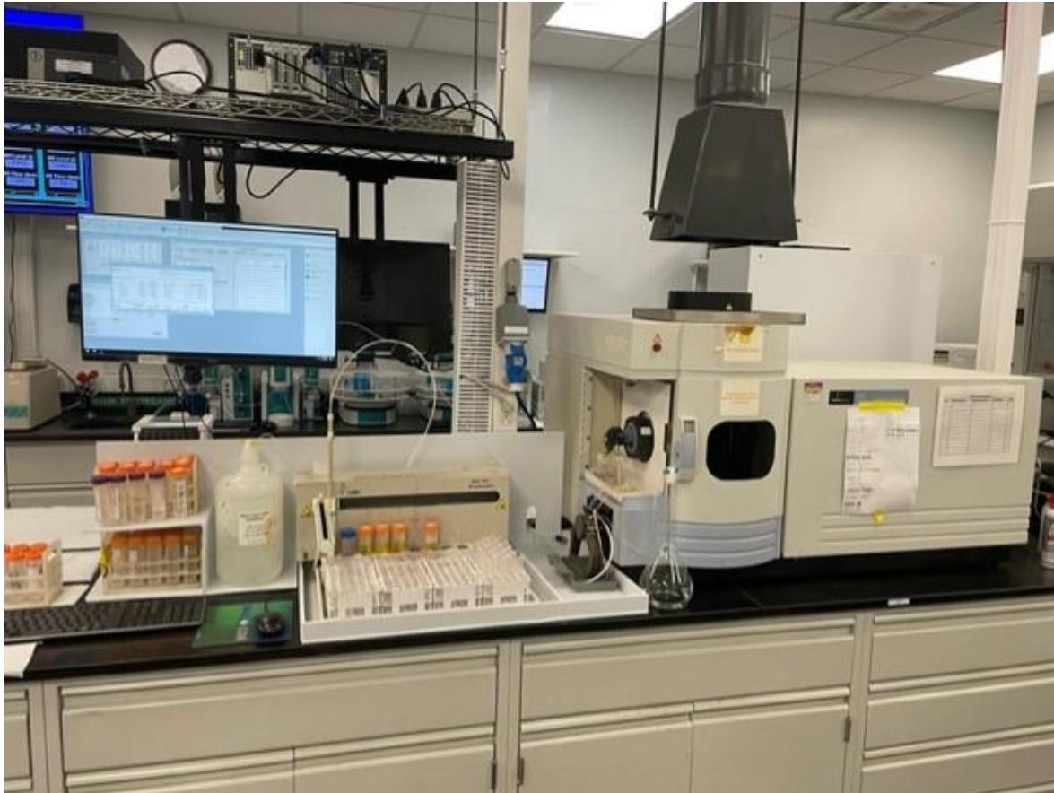
ICP-OES serves to quantify metals in solutions, offering the benefits of simultaneous multi-element analysis, heightened sensitivity, and a broader analytical range compared to atomic absorption (AA) spectroscopy.
