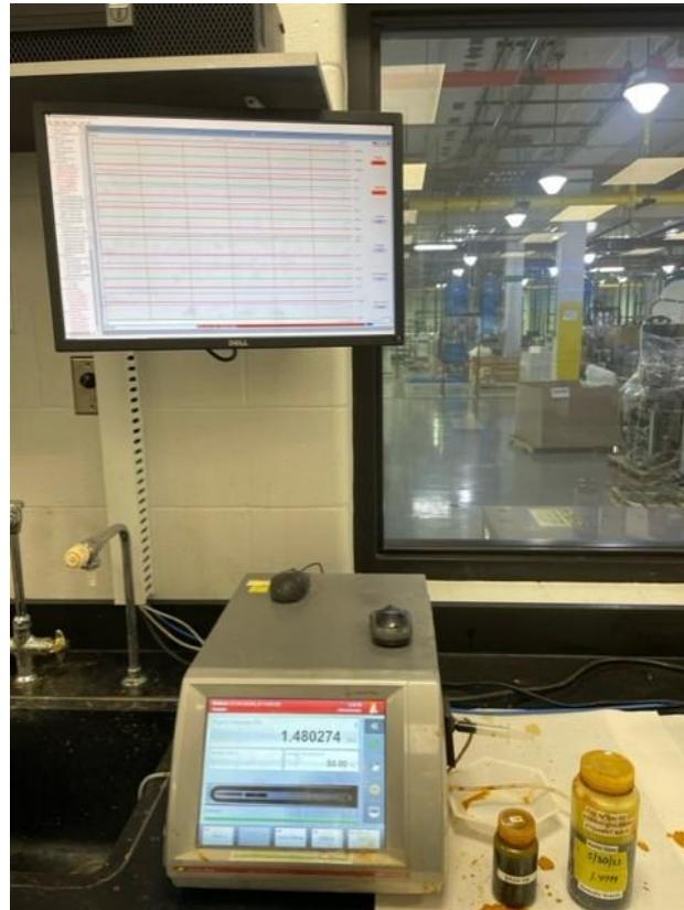
The DMA 4100 density meter boasts an accuracy of 0.00010 g/mL for density measurements and 0.02 °C for temperature readings.
