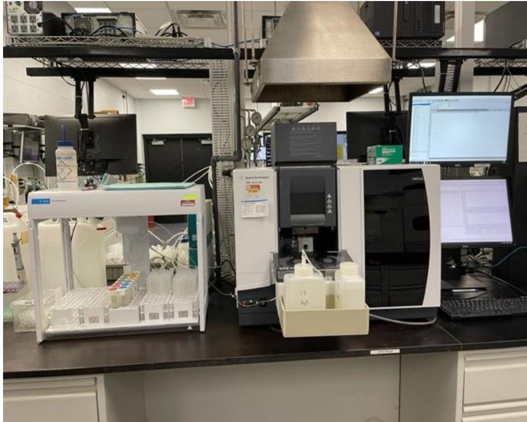
Atomic absorption spectrophotometry is a widely utilized technique for metal quantification across a diverse array of samples, capable of measuring both target and contaminant metals down to sub-microgram per milliliter concentrations.
