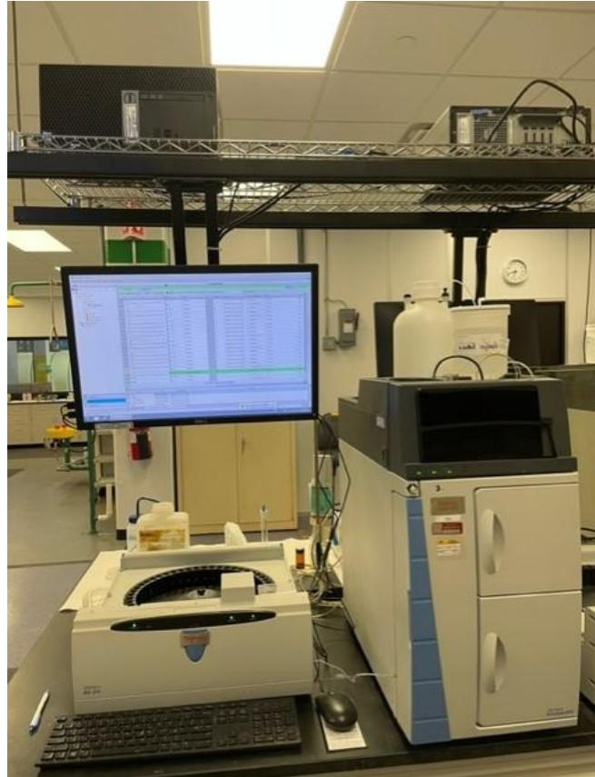
Ion chromatography is a high-performance liquid chromatography method that analyzes samples by separating and identifying ions or polar molecules. It is capable of measuring a diverse array of ion types across a wide concentration range.
