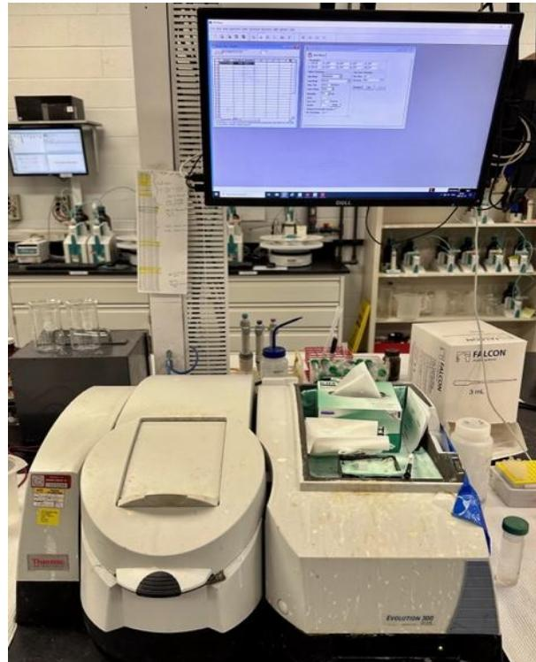
UV-Vis spectroscopy is an analytical method that quantifies the absorption of light by a sample across various wavelengths.
