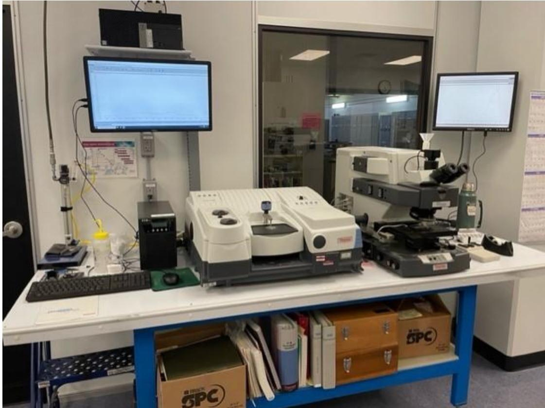
Fourier Transform Infrared Spectroscopy (FTIR) analyzes the absorption of infrared radiation by sample molecules, converting it into a unique spectrum. Interpreting this spectrum involves comparing peaks to reference data to identify molecular structures and functional groups, enabling substance identification and chemical analysis.
