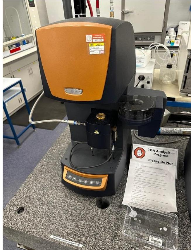
Thermogravimetric analysis (TGA) measures the mass of a sample over time as temperature varies, typically ramping from room temperature to around 1000°C. This provides insights into the sample's physical properties.
