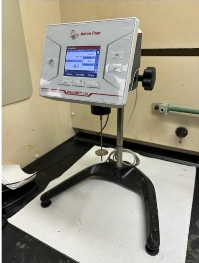
A viscometer is designed to measure the viscosity of materials within a range of 13 to 320 million centipoise (M cP), functioning by rotating a spindle at a controlled speed within the sample and quantifying the resistance as torque.
