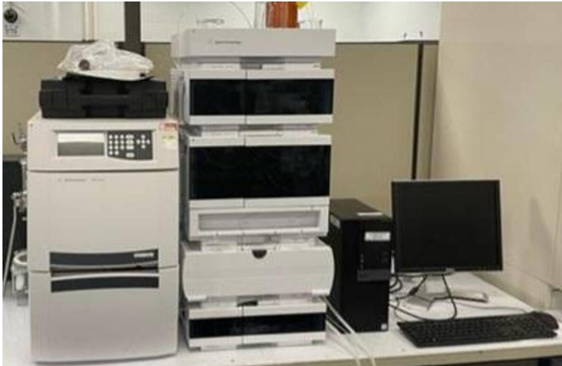
In Gel Permeation Chromatography (GPC), sample components separate based on their molecular size as they interact with a porous gel matrix. The eluted components are detected by a detector, generating a chromatogram. Interpreting the chromatogram involves analyzing peak retention times to determine molecular weight distribution and peak areas for quantification of component amounts.
