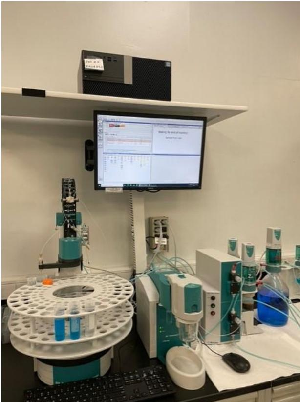
Cyclic voltammetric stripping (CVS) serves as a monitoring tool for the concentrations of organic additives in plating baths. It determines concentration by cyclically plating and stripping a sample.
