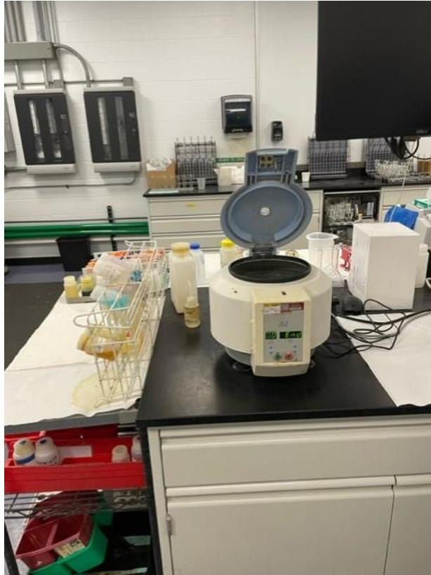
Centrifuges use centrifugal force, significantly exceeding gravitational force, to efficiently separate solids or precipitates from liquids. By rapidly spinning samples, they expedite the settling of denser materials to the bottom, enabling quick and effective preparation for analysis.
