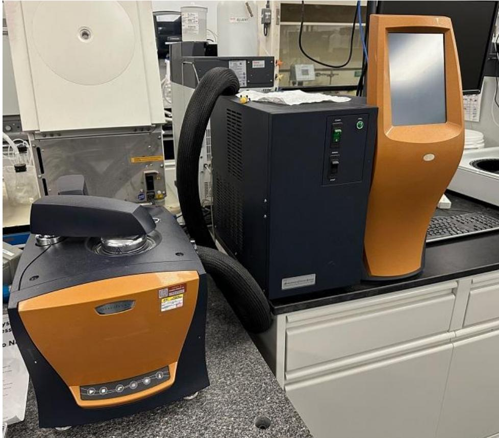
Differential scanning calorimetry (DSC) is a thermoanalytical technique that measures the difference in heat required to raise the temperature of a sample compared to a reference material, as temperature changes. It is commonly utilized for analyzing polymers and assessing oxidative stability.
