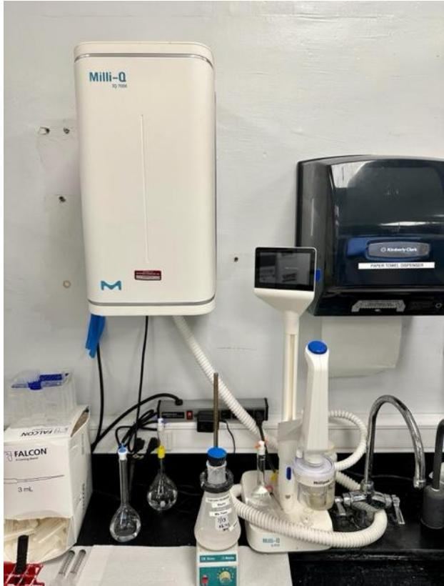
The pure water system employs an ion exchange resin to produce ultrapure water with a resistivity exceeding 18 MΩ·cm.
